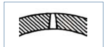
Keystone slot Cut under a 6° angle, this V-shaped slot is non-clogging.
