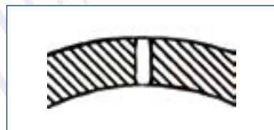
Straight slot Cut straight on the center, this conventional slot does not wear out.
